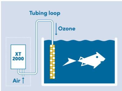
The ozonizer may be installed in an equipment cabinet. If the ozonizer is operated in a small enclosed space such as a cabinet, it is essential to provide sufficient ventilation to avoid overheating. If the ozonizer is installed below the water level, provide a loop of tubing extending above the water level to avoid water flowing back into the ozonizer.
