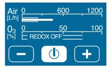
When using a redox controller, ozone production is turned off automatically once the target redox potential set on the redox controller has been reached. When the redox potential drops below the set value, ozone production is resumed.
