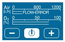
If airflow through the ozonizer drops below 75 litres per hour, ozone production will shut down to prevent overheating. Please provide sufficient airflow to the ozonizer, removing any blockages.
